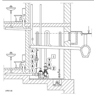
repair. The pressure pipe has to be passed above the locally defined backpressure level and a non-return valve tested in keeping with European standard 12050-4 has to be mounted. In keeping with European standard 12056 the ventilation pipe has to be passed up to the roof.
