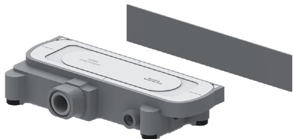
For free-standing installation, stick the enclosed insulation board onto the rear wall. Mount the four feet at the bottom of the tank and align the unit in height and horizontally.
