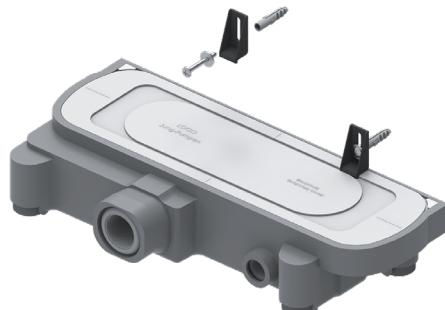
For wall mounting, use the enclosed wall fixing set to prevent
