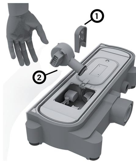
If the hydraulic system is blocked, pull the red fixing element upwards and take it out. Next, gently loosen the hydraulic system and remove it. After cleaning, make sure that when you re-insert it, the swing-type check valve and the two seals are firmly in place. To facilitate assembly, apply a little lubricant to the two sealing rings before fitting. Finally, the red fixation is inserted.
