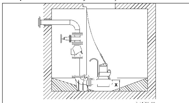
**Assembly:** Fix the coupling base firmly to the floor of the collection chamber using plugs and then mount the guide rails. Next, install the pressure pipe including the necessary fittings, such as the non-return valve and shut-off valves.
